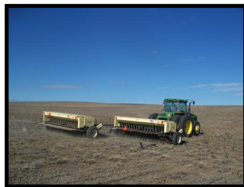
Figure 18. Multiple drill set-up being used to seed a 600 acre no-till field
