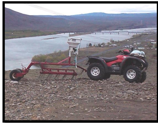
Figure 32. Spring-tine harrow with seed broadcaster mounted to frame.
