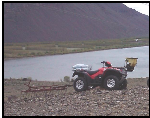
Figure 19. Truax seed slinger mounted on the front of an ATV, with a spring-tine harrow pulled behind
